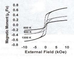
Fig. 1. Room-temperature VSM measurement result of CuO:Fe (2 at.%) powder for varying annealing temperature.
