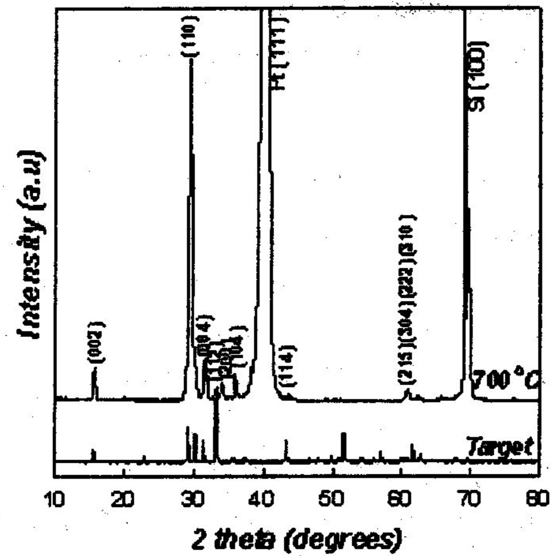
Fig. 1. XRD patterns for  $\text{HoMn}_{0.95}\text{Fe}_{0.05}\text{O}_3$  target and thin film.
